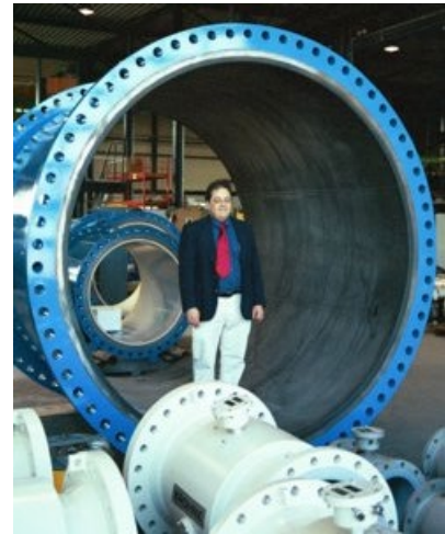
Dr. Yoder inside an 86-inch magnetic flowmeter
