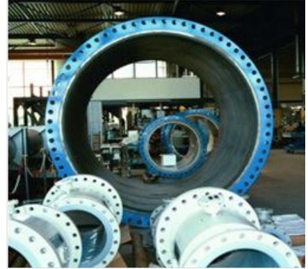
Magnetic flowmeters (Photo from Flow Research archive)
