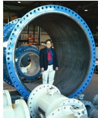
Dr. Yoder inside an 86-inch magnetic flowmeter
