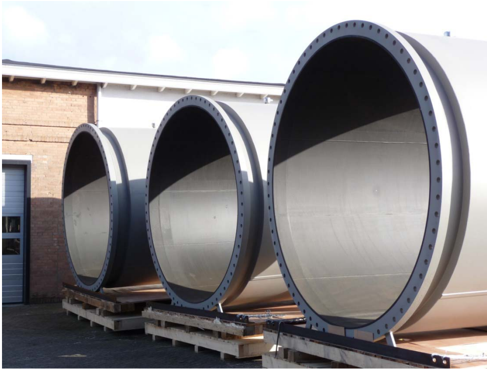
Three large diameter magnetic flowmeters await delivery.
