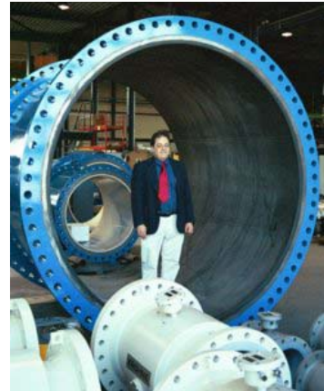
Dr. Yoder inside an 86-inch magnetic flowmeter
